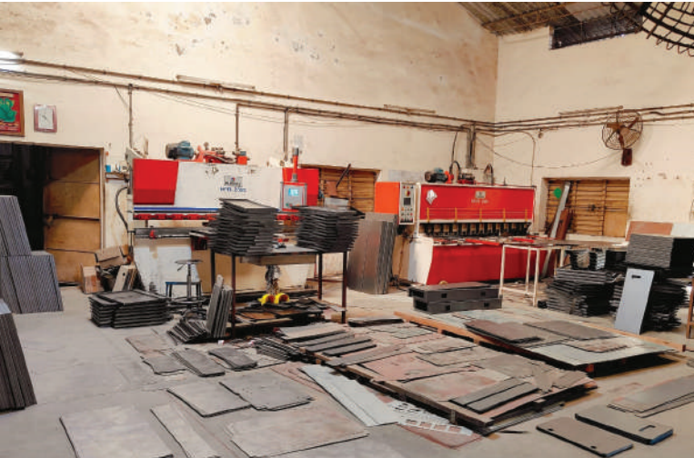
Bending of the components are done on semi automatic bending machines.
