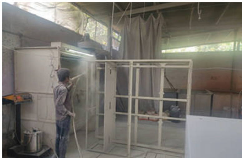
Powder coating is done by electrostatic process in spraying booth.
