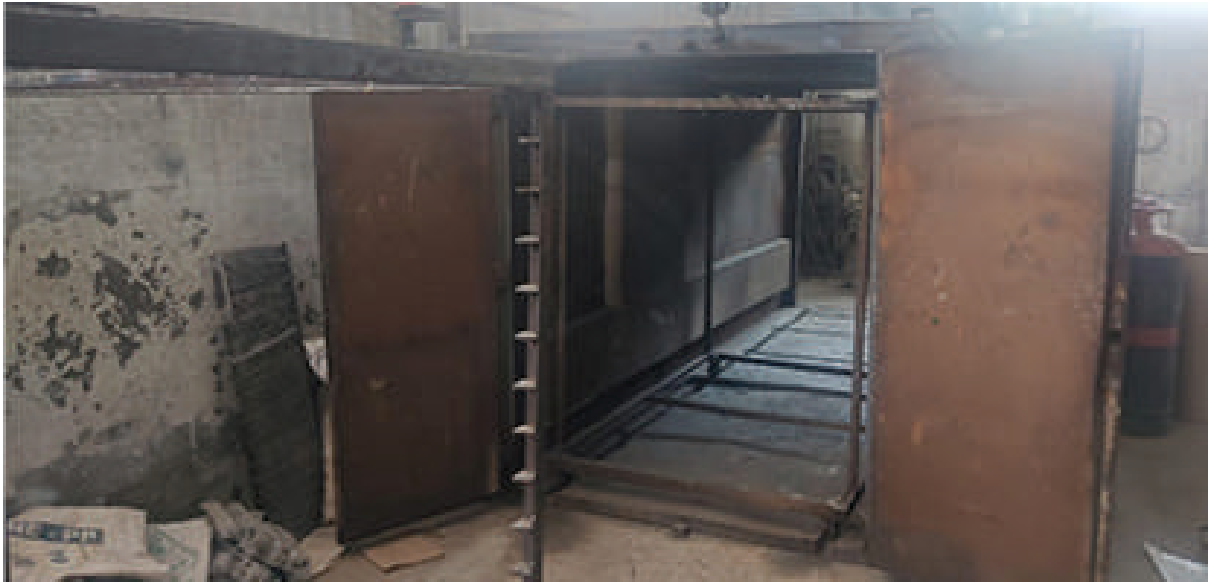
Powder coated components are cured in the oven to obtain smoother finish. (70-80 microns)
