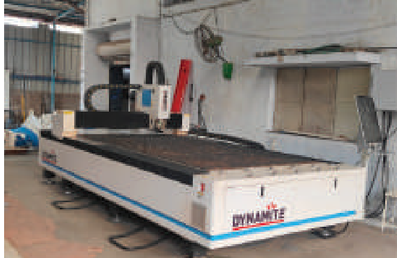
Sheet metal is cut into the needed component size on laser cutting machines.
