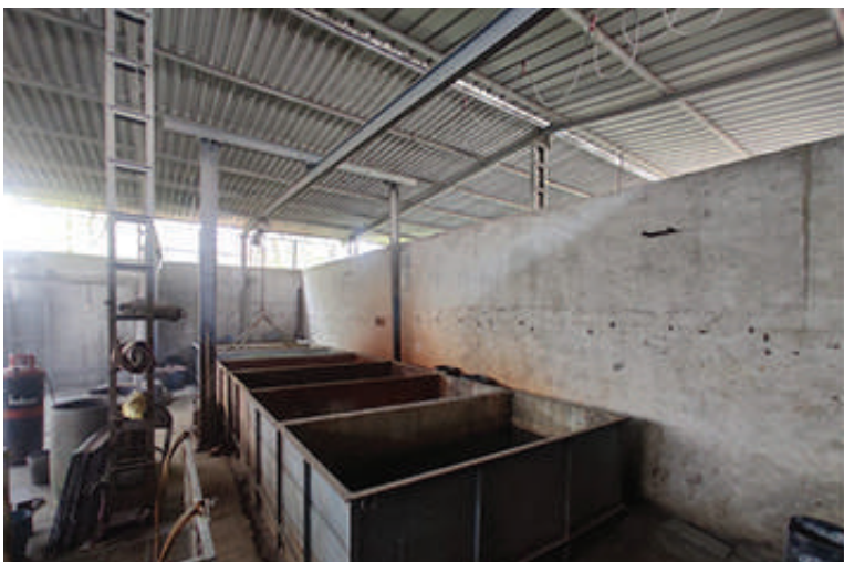
Seven tank pretreatment process is performed to ensure that components are ready for powder coating.
